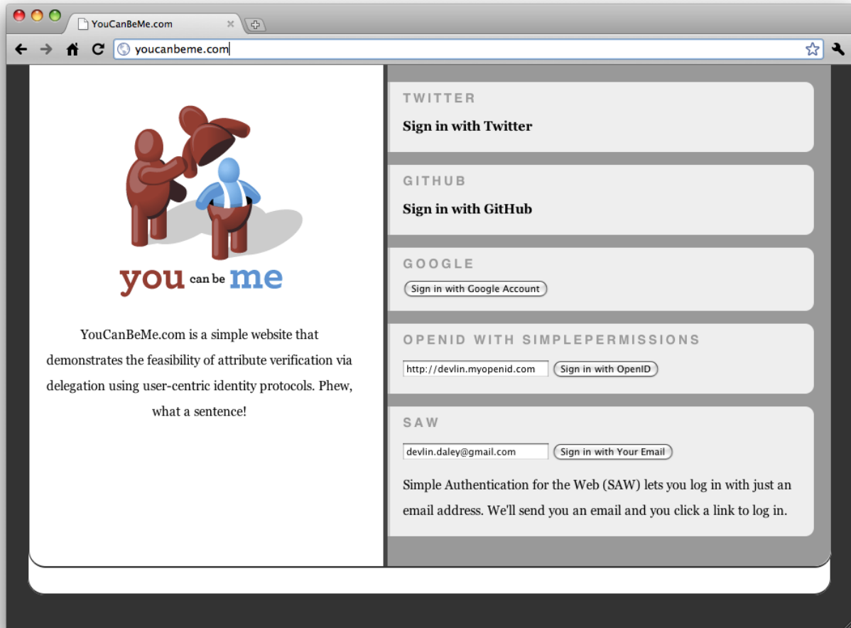
Figure 3.10: Login screen for YouCanBeMe, an identity proxy that furnishes selective delegation to OpenID that can be used for attribute verification.
